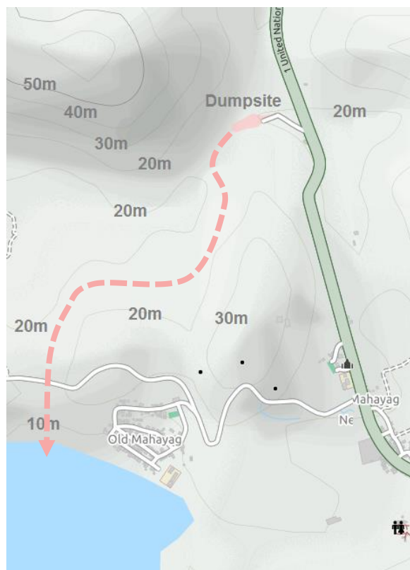
Figure 6. Most likely route of leachate runoff during heavy rains
