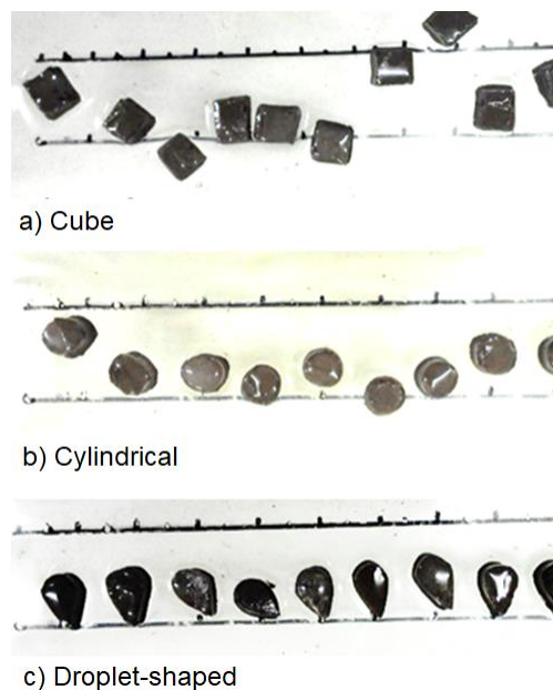
Figure 5. Displacement of Model Rock Mounds After Wave Exposure (One Row)
