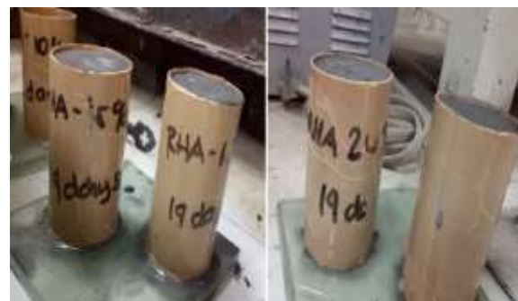
Figure 1. Sample Specimen (50ø x 100mm) 3.4 Testing Facilities and Procedure
