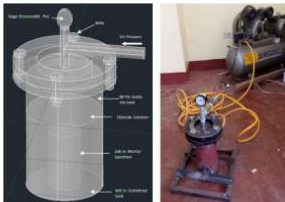
Figure 2. SSU Solution Penetration Apparatus
