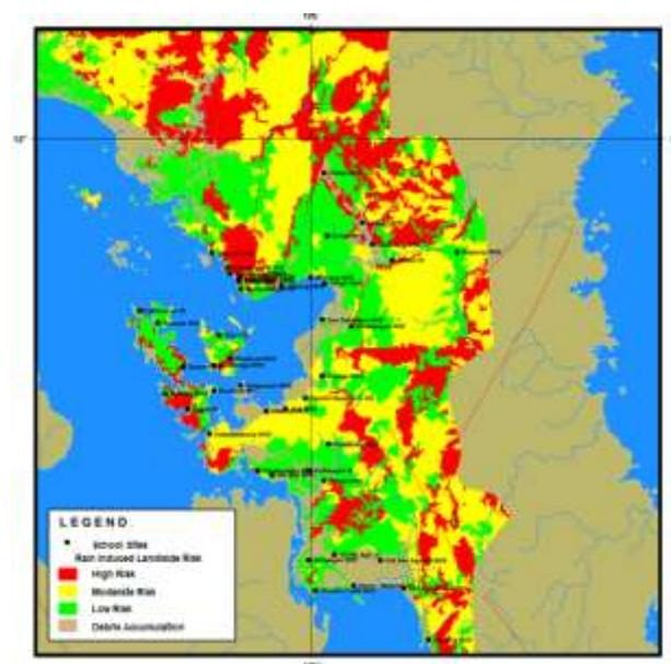
Figure 9. Rainfall-Induced Landslide Exposure of School Buildings
